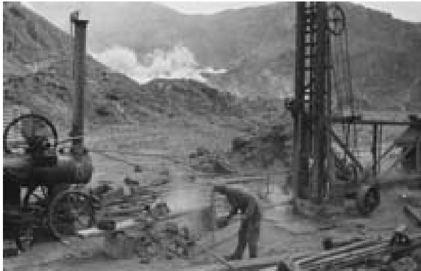
Photographer unidentified, White Island Products sulphur extraction enterprise on White Island, showing a plant worker in the foreground, and a stationary steam engine driving extraction machinery [Between 1925 and 1930]. Alexander Turnbull Library, Wellington, N.Z. F- 59931-1/4.
